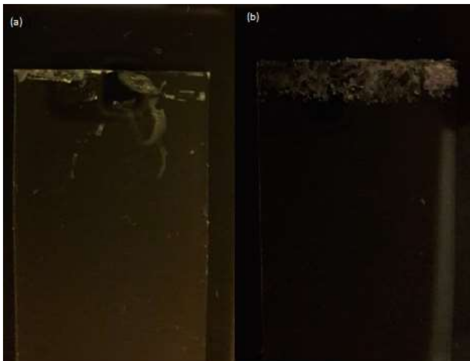
Figure 33: (a) Zn-film at C=1.4\text{ M} leaves an inhomogeneous film layer (b) Zn-fil at C>2.3\text{ M} is inhomogeneous but the solution was supersaturated, which means the concentration is too high
