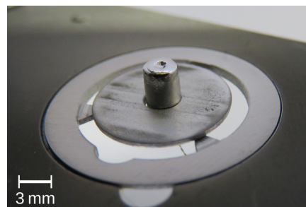
FIG. 7. Photograph of a Ti source after approximately 300 nm of Ti was deposited on the substrate. The surface has melted, generating a dip at the location of the laser spot. The structural integrity of the source has remained intact.
